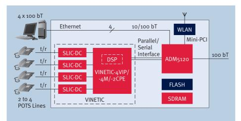
VoIP Router and ATA Application Example for One Hardware for All "Voice over Packet" Applications
